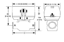
Fig.4 – 3-way nominal dimensions in inches and millimetres
